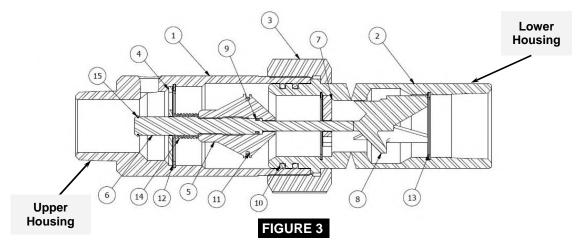
3. When the SB100/125 is fully engaged, the Upper Housing (1) is secured to the Lower Housing (2) by Lock Nut (3) The separation is accomplished when, and only when a pull away occurs.
