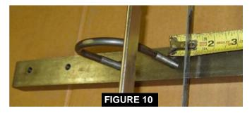
7. Install the Shear Securing Bar with appropriate u-bolts, nuts and lock washers as shown in Figure 11. \*Make sure to tighten bolts firmly.\*
