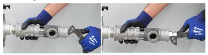
**Step 1:** Slap the Valve Handle (a) to the CLOSED position (a). Ensure the Safety Handle Latch (b) is engaged into the bonnet slot (c). This prevents opening of the Valve if the handle is struck accidentally.
