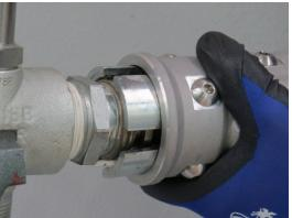
Step 3: Release the Locking Collar ② and allow the Collar spring to close the Acme Jaws, rotate the Collar slightly clockwise until the jaws snap into the Male Acme Threads.
