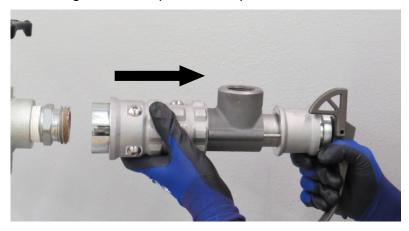
Step 2: With the Acme Jaws held open, place the Acme Jaws over the Male Acme Connection until the Seal Face ⓐ is resting squarely on the rubber seal of the Male Connection.
