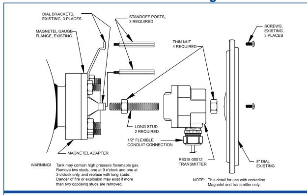
NOTE: This detail for use with centerline Magnetel and transmitter only STANDOFF POST, 3 PLACES DIAL BRACKET, 3 PLACES MAGNETEL GAUGE FLANGE LONG STUD, 2 PLACES ⊕ INNER NUT, 2 PLACES OUTER NUT, 2 PLACES (O) R6315-00012 TRANSMITTER 8" DIAL
