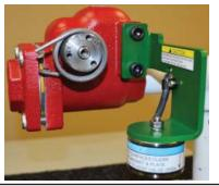
NOTE: Position of 3 holes on the Return Spring Arm.
