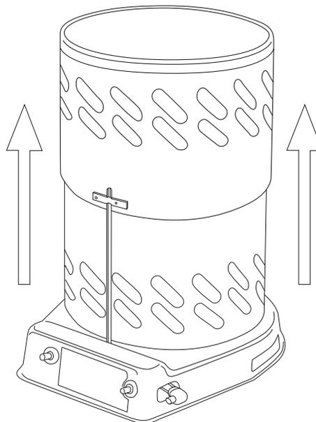
STEP 2: LIFT OUTER SHELL STRAIGHT UP. CARE MUST BE TAKEN TO PROTECT HANDS DURING LIFT.
