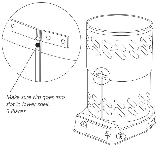
*Make sure clip goes into slot in lower shell.
