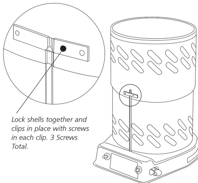
*Lock shells together and clips in place with screws in each clip. 3 Screws Total.*
