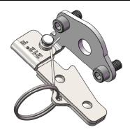
cap screws). The new cover plate / latch assembly can be attached to the internal valve with the retained cap screws. Tighten the screws to 25 to 30 inch pounds / 2.8 to 3.5 N•m torque.
