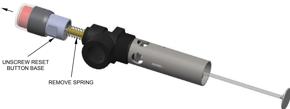
Figure 11B – STEP 2 – Unscrew reset button base and remove the spring
