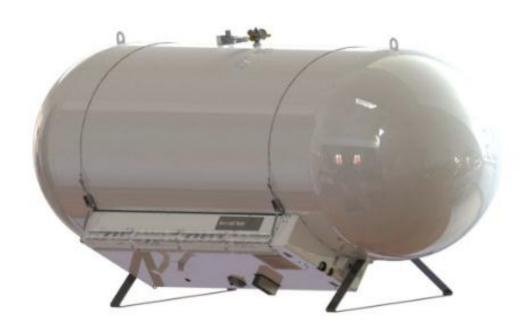
A solid state thermo-electric generator provides power to operate the tank heater controls. Electrical power is generated by the temperature differential between the heater and the ambient air. The small finned aluminum heat exchanger cools one side of the EMF generating device, and the heater provides heat to opposite side. The heat exchanger must remain exposed and unobstructed. A common "flame type" thermocouple does not function in this application because there is no pilot flame.
