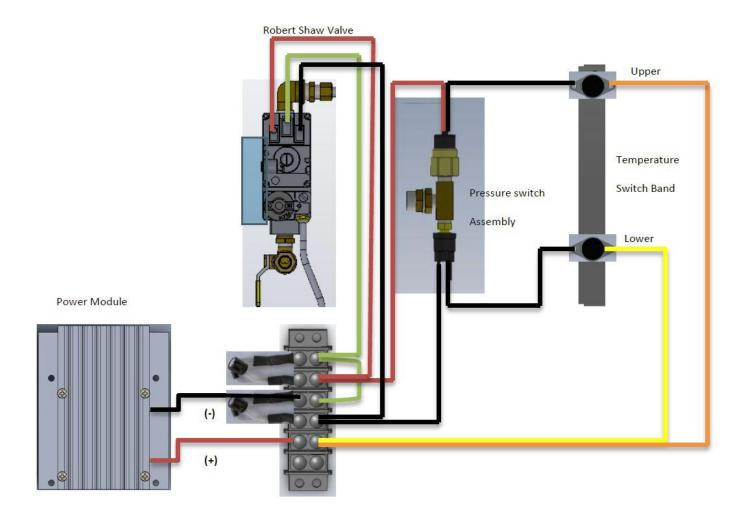
Figure 11: Adjustable pressure switch settings
