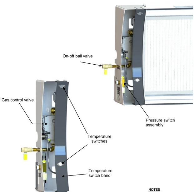
1. WHEN INSTALLING THE TANK HEATER MAKE SURE THE TEMPERATURE SWITCHES ARE MAKING FULL CONTACT WITH THE TANK SURFACE. FAILING TO DO SO WILL TRIGGER THE TEMPERATURE SWITCHES AND KEEP THE HEATER FROM MONITORING TANK SURFACE TEMPERATURES PROPERLY.
