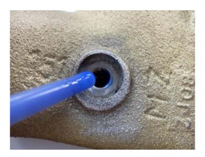
3. Slide pin gasket (P/N 8135-101) over the pivot screw (P/N 3-4169) threads as shown in the picture.
