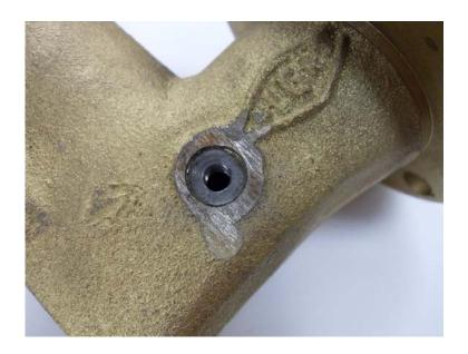
2. Apply blue (medium strength) Locktite 243 or Permatex to threads on the liquid inlet valve body or pivot screw.
