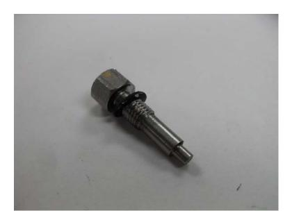
4. Screw in pivot screw to the inlet valve body and apply 8 in-lbs of torque (approximately 1/8" full turn).
