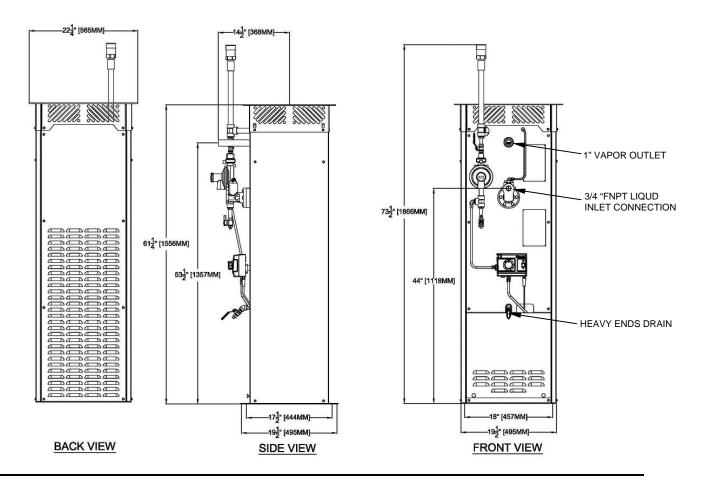
Figure 3 - Installation - 160H vaporizers
