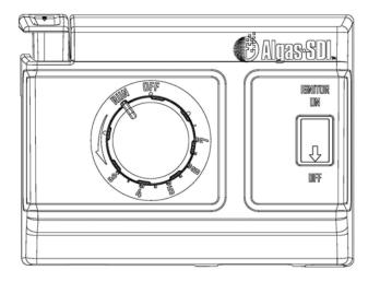
5. Turn the igniter switch to "ON". Press the pilot button. Continue to hold the pilot button for 30 to 60 seconds and release. Pilot should remain lit.
