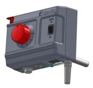
2. Pull out the battery, disconnect it and replace with new 9VDC battery. Push the battery back in the thermostatic gas valve housing and close the battery access door prior to turning the reignitor switch ON.
