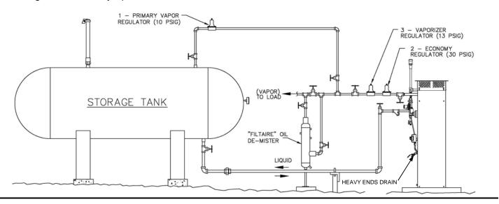
After installing the vaporizer, install and set the regulators from the economy kit as follows:
