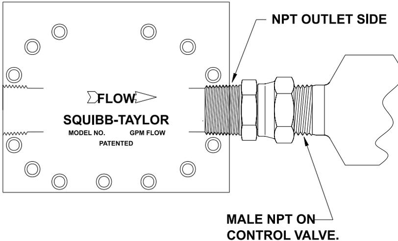
A Swivel Connector is provided for installation into the Outlet Side of the Kontrol-Flo Meter Body. Check Flow Arrow on the cover for proper orientation. Using Teflon tape or pipe dope, install the male pipe thread into the Meter Body. Do not over tighten.
