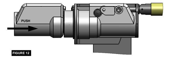
6. Screw the handle in until its snug with washer/bracket to engage the handle with the bracket Actuate cam action by pivoting the bracket handle 80-90 degrees, as shown in figure 13, push the Male Plug in, which will allow the Male Plug to move to its operating position and the Latch Balls to engage.
