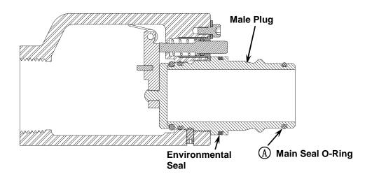
5. <u>Make sure the Bleed Valve is open</u>, then insert the Male Plug into the Female Socket as far as possible using only hand pressure. As shown in Figure 12.
