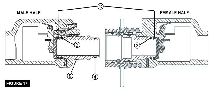
If the Plunger or Plunger O-Rings become damaged, a Service Kit is available through your local distributor.
