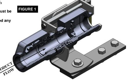
1. When the Flo-Max II Coupler is engaged and under pressure, the spring-biased Inlet Swing Check ① is held open by the Plunger ②. The spring-biased Outlet Swing Check ⑤ will be opened when NH<sub>3</sub> flow begins.
