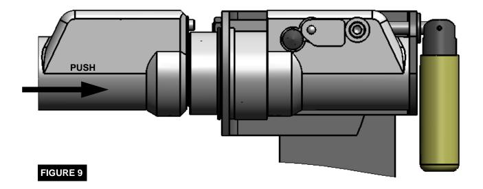
7. Screw the handle in until it's snug with washer/bracket to engage the handle with the bracket. Actuate cam action by pivoting the bracket handle 80-90 degrees as shown in Figure 10. Hold in this position and push the Male Plug in, which will allow the Male Plug to move to its operating position and the Latch Balls to engage.
