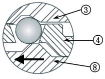
DETAIL "Y" Male Plug ⑧ starting to disengage from Female Socket ④ allowing full disconnect.
