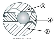
DETAIL "X" Male Plug ⑧ installed in Female Socket ④ in the engaged and operating position.
