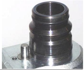
17. Place the Retainer over the threaded hole, secure with the Cap Screw, and tighten with the 5/32" Allen wrench.
