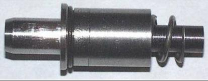
13. In order to keep the Spring from falling off, hold the Plunger Assembly at an angle and install it into the Male Body.
