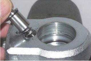
14. Make sure the top of the Housing is just about flush with the face of the Body. **NOTE: If the Housing is not flush with the face, remove the Plunger Assembly and repeat steps 12 thru 14.**
