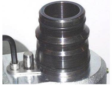
18. **Taking care not to damage the Plunger, tighten the Male Plug with a large adjustable wrench.**
