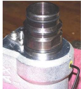
20. The manufacturer suggests that an air test be performed on the entire assembly prior to returning to service.
