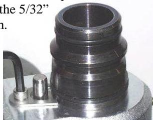
8. **Taking care not to damage the Plunger, tighten the Male Plug with a large adjustable wrench.**
