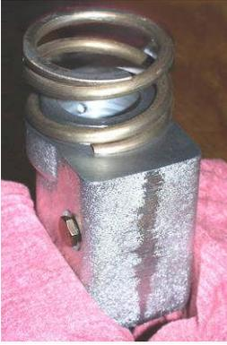
7. Lightly lubricate the Ball Carrier threads with a non-petroleum based lubricant.
