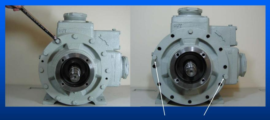
Remove the head bolts. There are threaded holes that may be used if needed to "push" the head off of the casing. If just changing a seal the head does not have to be removed.
