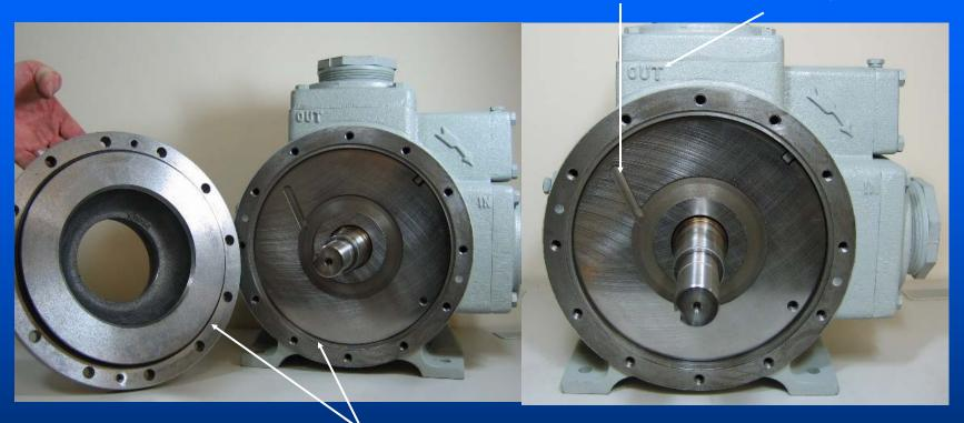
The head may be removed and the O-ring area of the case and head should be cleaned before assembly. On the 1021 and 1521 the sideplate has a groove that must be directed toward the discharge side of the pump. If the plate is reversed it must move to the opposite side.
