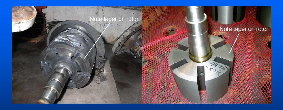
The Rotor/Shaft assembly normally does not need to be changed. It usually is only damaged if foreign material is ran through the pump or if the bearings are not maintained. The rotor has a "taper" towards the outside diameter. If the taper can still be seen, the shaft is probably re-usable.
