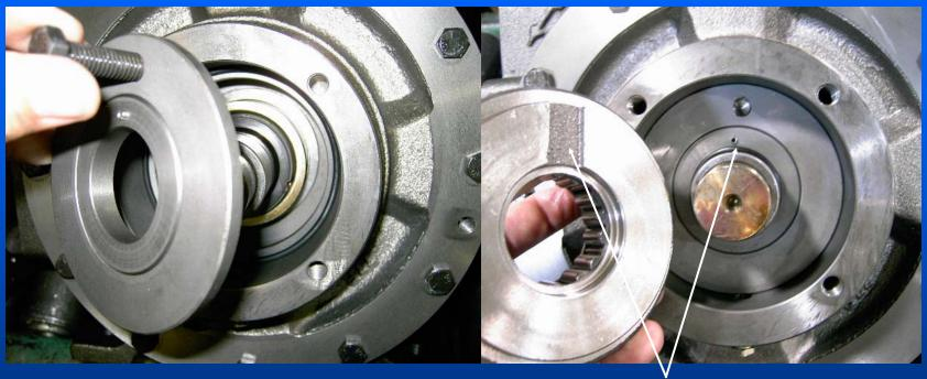
Install the seat in the seat adapter and carefully install the assembly over the shaft. Take care not to hit the seat against the shaft. Using a spray lubricant to rinse the faces will assure the surfaces are clean.
