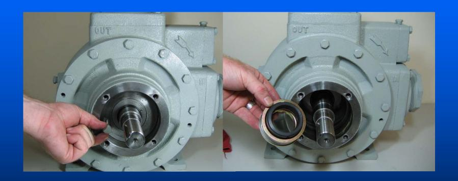
The inside of the head and the shaft should be cleaned before installing a new seal. The seal may be lubricated with a light oil or spray lubricant during assembly. Seals are precision parts and care must be taken during handling. **KEEP HANDS CLEAN!**
