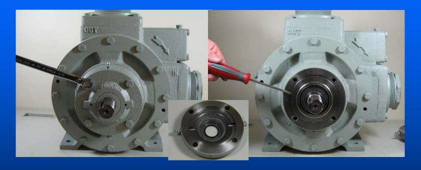
Before any repairs, confirm all pressure has been relieved. Remove the bearing cap bolts and bearing cap. The grease should be cleaned from the bearing cap and the grease seal removed and replaced. The bearing housing may be removed with one or two screwdrivers using the groove on the diameter of the housing to pry out the housing. If the housing is difficult to remove the head may be removed and using a rubber hammer or piece or wood, drive the housing out from the back.
