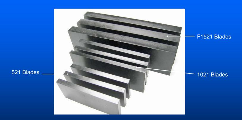
Standard 521/1021/F1521 pump blades are of solid design and may be reversed or flipped if any chipping or damage is noted. The blade should be changed when more of the blade is extended out of the rotor slot than is remaining in the slot. See the IOM manual for more dimensions.
