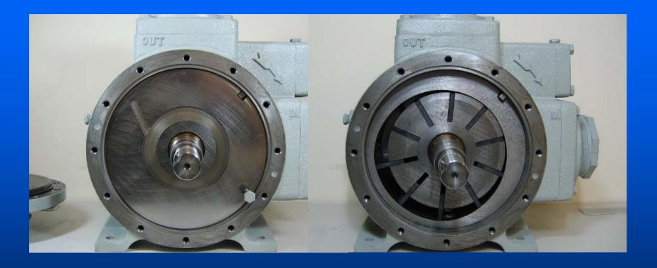
The sideplate can now be removed using a head bolt to assist. This allows access to the inside of the pump for inspection of the blades and cam.
