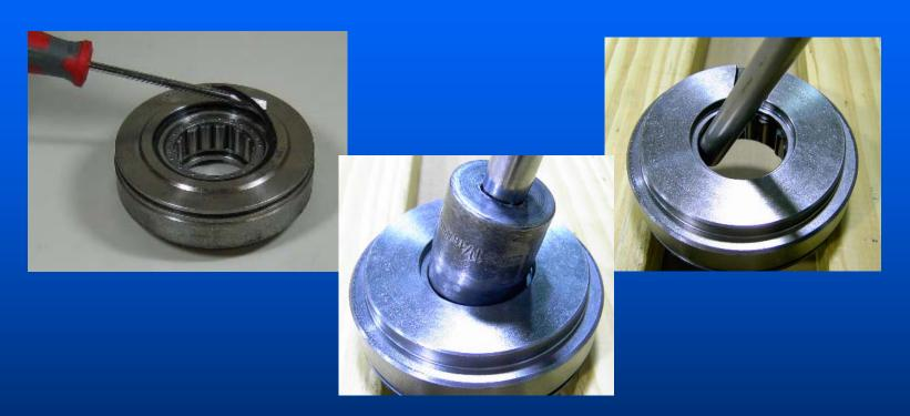
The main bearing can be removed by removing the spiral retainer ring and pressing the bearing out. A tool such as a socket or punch may be used to drive out the bearing. Both the inner and outer bearing should be changed together. The bearings may be "pre-packed" with grease during assembly, but it is not required.
