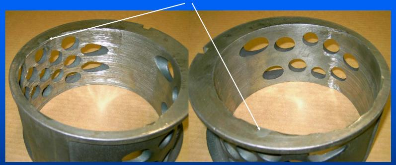
The above cam is severely worn due to the improper installation of the sideplates. The sideplates had been reversed, but had not changed sides placing the feeder channel towards the suction. This position maintains a low pressure behind the blades causing the blades to move back into the rotor slots instead of holding against the cam inside diameter.
