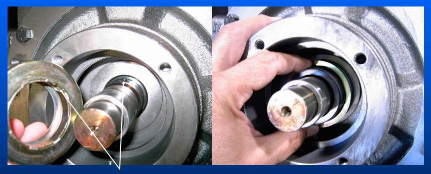
Clean the shaft surface were the O-ring seals prior to installing the spring When installing the seal it is easier to install the spring retainer first, watching the seal pin alignment.
