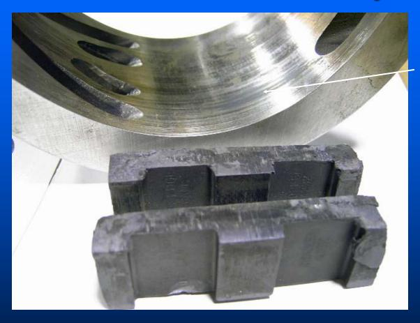
Melted blade material in cam Inside diameter.
