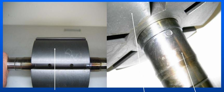
Inspect rotor outside diameter for scoring and wear. Wear in this area is typically caused by foreign material such as rust welding slag, etc.
