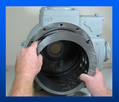
The cam may be removed by using a pieces of hardwood and tapping around the outer edge of the casting. The cam should be inspected for wear and scoring on the inside diameter. Small scratches seldom reduce pump efficiency, but if deep grooves are present the cam should be changed. "Washboard" type wear is usually caused by cavitation and the cam should be replaced.
