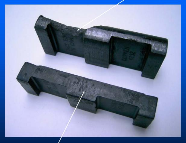
Blade damaged from "dry" running, and melted.
