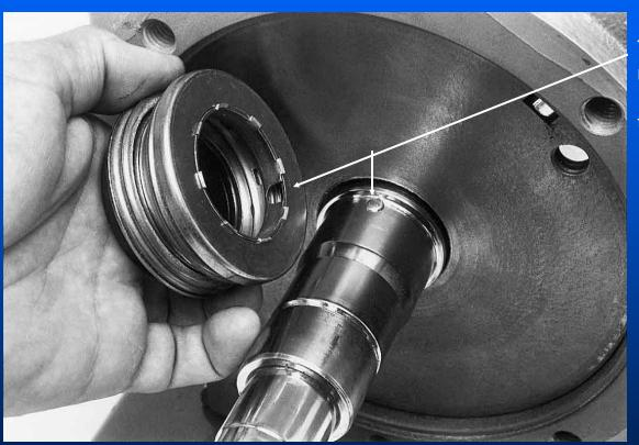
The seal spring has a notch that must align with the pin on the shaft. It is best to install the spring first, then install the carbon and O-ring.
