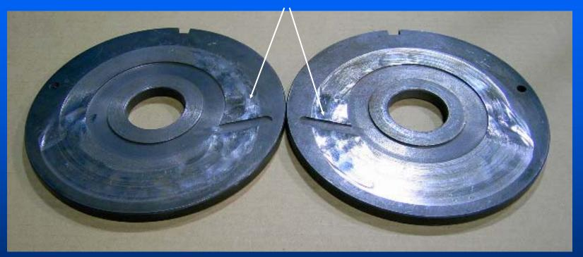
Scoring on sideplates may be caused by foreign materials such as rust, welding slag and other materials being pumped. Light scoring will not typically reduce pumping performance. Sideplates may be reversed or "flipped over" on all models except the F/T1521. Care should be taken to maintain the feeder channel toward the discharge side of the pump. The 1021 plates must change pump sides to be reversed.
