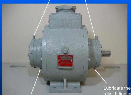
Lubricate the bearings only until the relief fitting pin moves.
