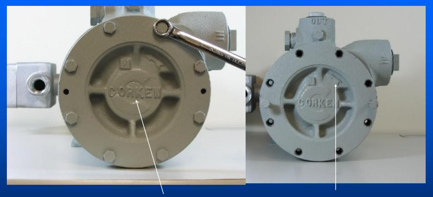
Remove the cover bolts and use two bolts to "push" off the cover if necessary. Note cover position and direction arrow. The pump operates "CCW" when facing the cover.
