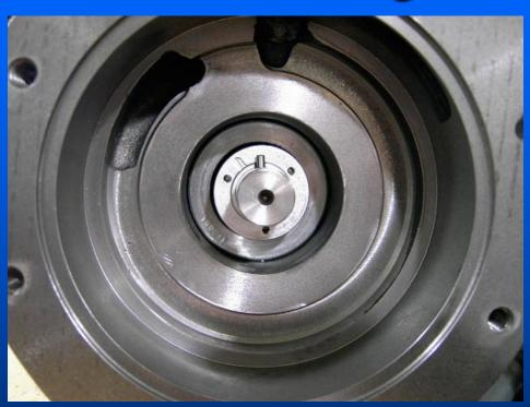
Normally a pump is rebuilt using the same housing shims. To confirm proper clearance:
