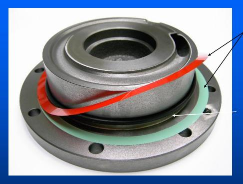
Shims are for adjusting impeller clearance. Red =0.002 inches Green = 0.003 inches Proper clearance = Approx. 0.003 inches max.
