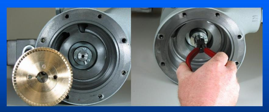
Once the impeller is removed the special key must be removed. A pair of "side-cutters" is an easy way to remove the key. This can be done by gripping the key and and applying upward pressure on the side-cutters. This can also be done with a small screwdriver inserted under the "tab" on the special key. Care should be taken to avoid damage to the shaft.
