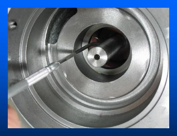
Remove the casing O-ring using a pick or probe. Once the O-ring is removed, clean the groove using a spray lubricant or air to remove any particles that may have fallen into the groove.
