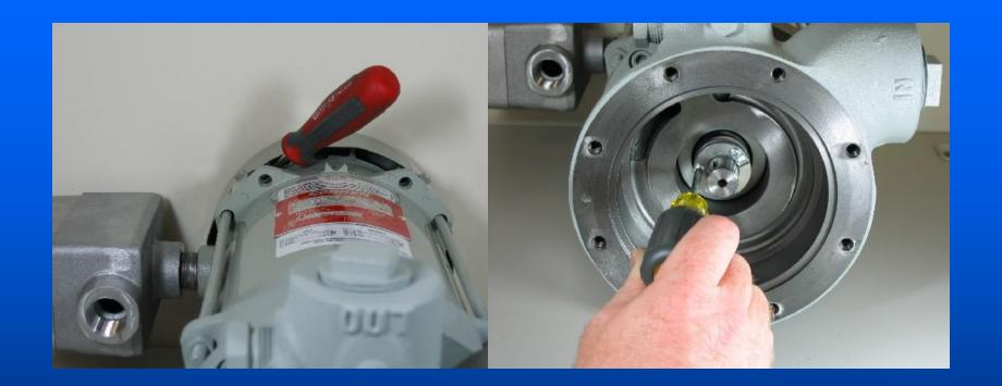
Insert a screwdriver into the motor fan on a "C" model or lock the shaft on a DS, DL or F model pump to remove the seal clamp ring screws. The screws not only hold the pin, but also compress the sleeve O-ring to the shaft. They should be tightened during assembly, taking care not to strip the threads. A screwdriver or other tool should also hold the shaft during assembly.
