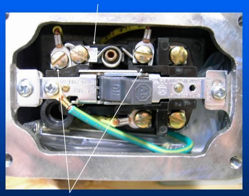
On 115V the wire leads are on either side of the heater for C10-C13. If both wires are connected to one end it will trip over-loads.
