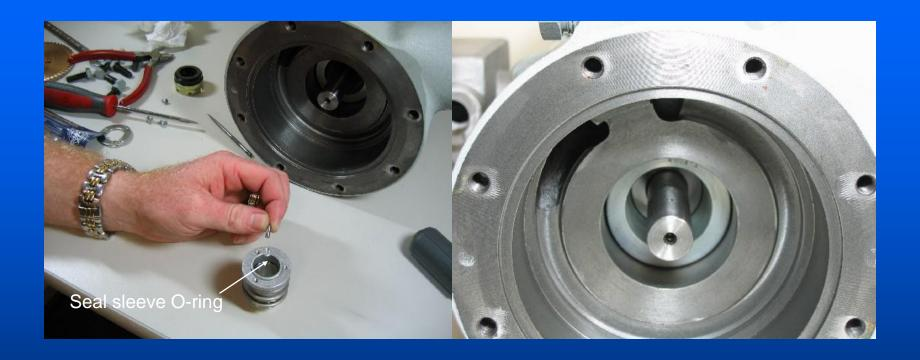
The seal sleeve should slide out easily. If it is difficult to slide off of the shaft, the shaft should be polished to remove any burrs around the pin hole or keyway to allow easy assembly. This can be done using a fine sandpaper or polishing cloth. The shaft should also be cleaned where the sleeve O-ring contacts.
