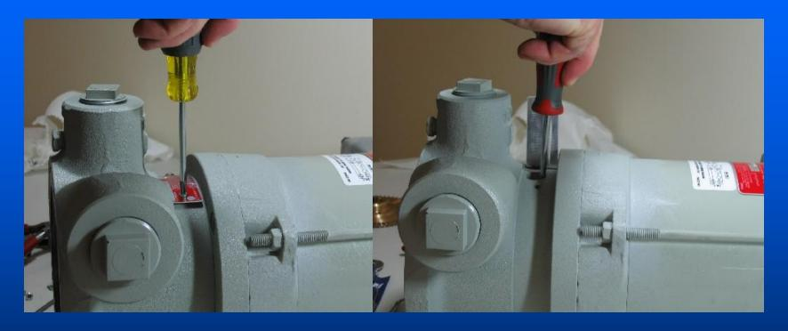
To remove the seal housing it is necessary to remove the nameplate. Then using a large flat blade screwdriver, pry outward on the housing. The screwdriver is prying on the grooves on the outside diameter of the housing. Holding up on the housing from the inside may assist in the removal.
