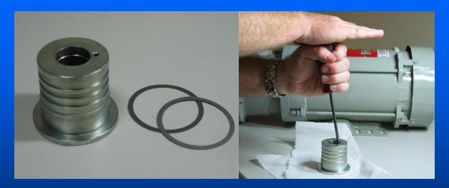
The above photograph shows the housing shims and the removal of the seal seat. These shims must be reused and do not come with a seal assembly. The housing should be cleaned on the outside and inside diameters prior to re-assembly.
