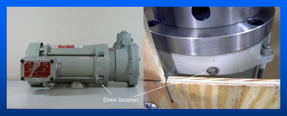
Explosion-proof motors "breath" and can accumulate moisture. Model C10-C13 pump motors include special drains to help eliminate this problem. Due to the applications most motors run intermittently. To avoid accumulating moisture, periodically operate the pump for 10-15 minutes straight. This will assist in evaporating the moisture. See "Engineering Data" page ED200 for more information.
