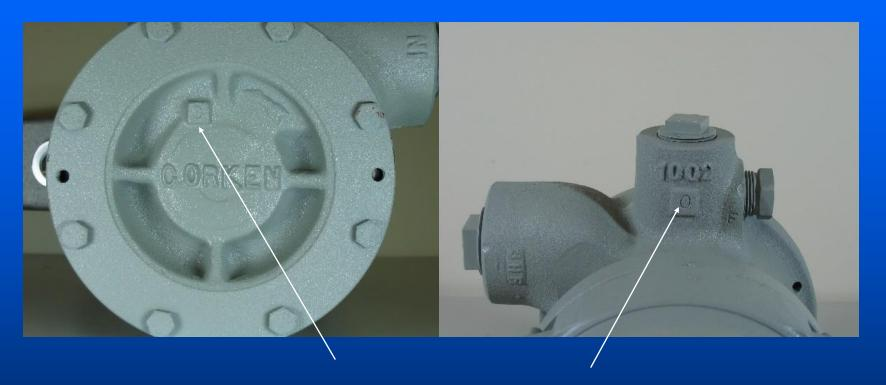
If the nameplate is missing the pump size can be determined by confirming the number stamped on the case and cover. This is a model "10", so you see a "0" stamped. A model "12" would have a "2", a "13" would have a "3", etc.
