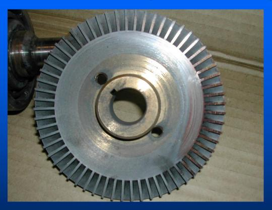
When an impeller is dis-colored such as shown in this photograph, the pump has operated "dry" or without liquid. This can be the cause of a seal failure. Inspect the system, bypass setting and operation to determine the cause of dry running. Note, the impeller may not be damaged if it can be properly shimmed and no "fins" are bent or damaged.
