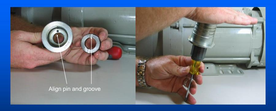
The seal seat should be installed using the "protective" cardboard disc supplied with the seal assembly. This can be done using a wood or plastic handle of a screwdriver or hammer and pressing in by hand. The seal and O-ring may be lubricated with a light oil or spray lubricant. Take special care if dirt or dust is present in the area. The seal is a precision part and debris may cause a leak. **Keep hands clean!**
