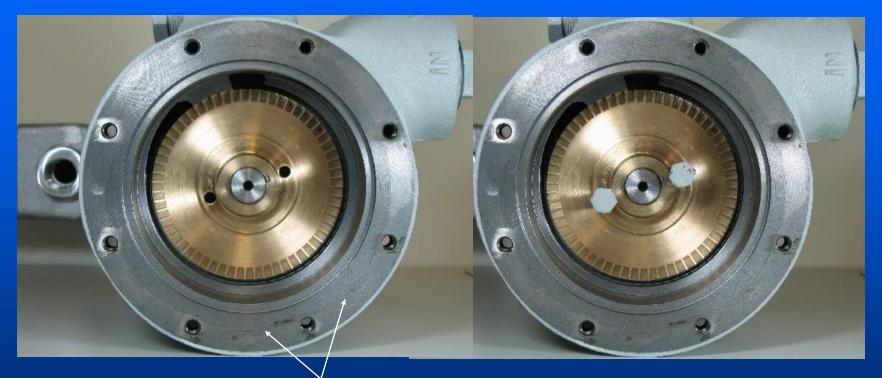
Cover has been removed. The flat case surface should be cleaned prior to re-shimming the impeller clearance.
