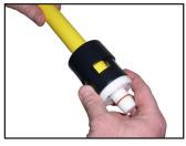
4b Chamfer end of pipe using Continental's double ended ID chamfering tool.
