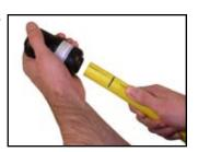
6 If using ID chamfer tool with gauge, check for proper chamfer by inserting pipe on gauge up to the oring. With proper chamfer, oring will begin to enter pipe.
