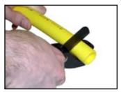
Chamfer end of pipe using Continental's double ended ID chamfering tool.
