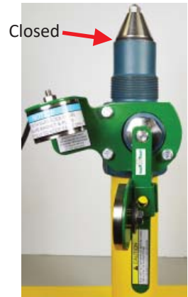
Power Off & Valve Closed.
