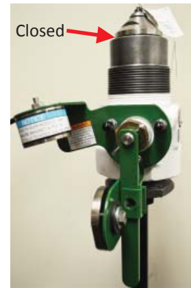
Power Off & Valve Closed.
