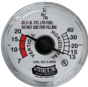
403582 - 33 1/2# Dial Snap-On V = 7-20% H = 13-40% Lift Truck
