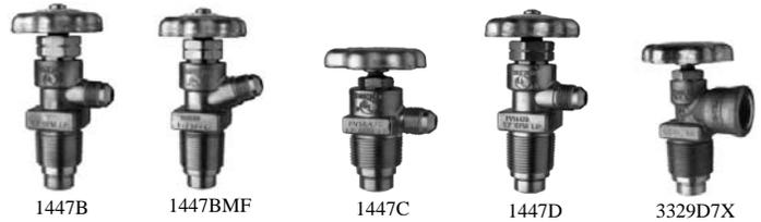
The **1447B**, **1447BMF** and **1447C** (Low Profile) valves have an excess flow check at inlet. Designed for withdrawals of liquid from engine fuel containers that contain a separate relief valve. The **1447D** has an excess flow check at inlet, plus an internal hydrostatic relief, which vents trapped liquid with excessive line pressure back to the tank. **3329D7X** is a vapor service valve with excess flow check.
