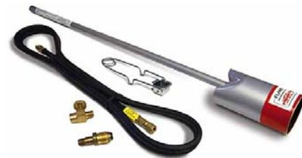
**JET 8** Head Mix Torch - Twin vapor flamer features up to 1.7 million BTU and plenty of length, a great combination for those big jobs which require high heat. The twin burners mix at the torch head reducing the risk of flashback at the handle. Flame length up to six feet.
