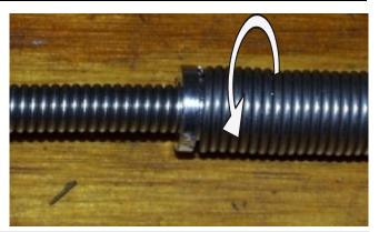
**32.** Unpack the Spider Adapter from the kit, install it over the Extension Cable and thread it into the Large Sheath turning **counter-clockwise**.
