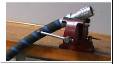
7. Using the pliers, pull the Cable Clamp outward and loosen the socket head cap screws with the 3/16" Allen wrench. As the second screw is loosened, the Cable Clamp will be free to slide off the end of the cable.
