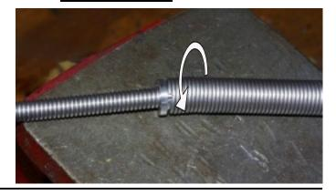
**18.** Re-install the Outlet Housing onto the end of the new hose that the PR4 is being transferred to, with the two 18" Pipe Wrenches positioned as shown.
