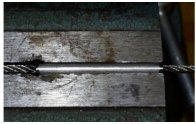
31. Re-install the Large Sheath on the threaded portion of the Sheath Adapter by turning <u>counter-clockwise</u>.
