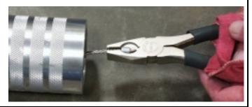
**3.** Secure the Outlet Housing and pull the cable outward until you feel the Poppet release to it's "tripped" position.
