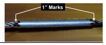
**30.** Carefully place the Cable Connector, with both Cables installed, into the jaws of a bench vise. Be sure each Cable is still inserted 1" into the Cable Connector and tighten the vise. The Cable Connector will be flattened and will grip the Cable ends tightly.
