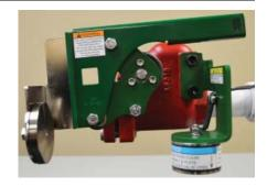
6. Rotate Handle counterclockwise to open valve. Strike Plate should latch against Surface of Electromagnet and stay attached to the Surface of Strike Plate while voltage is applied. Valve must stay open. Upon de-energizing the Electromagnet, the Handle and Valve must quickly "snap" closed. The Handle and Valve must quickly rotate and close either when (a) the power source is turned off or (b) the handle is pushed closed from the latched open position.
