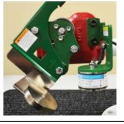
Connect electromagnet to the 12 V DC system and turn on voltage to the electromagnet.
