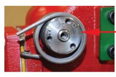
NOTE: Position of 3 holes on the Return Spring Arm.
