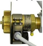
Slide sensor assembly forward on barrel of ME868 Series Acme adapter until face of sensor body touches back of flange on Acme
