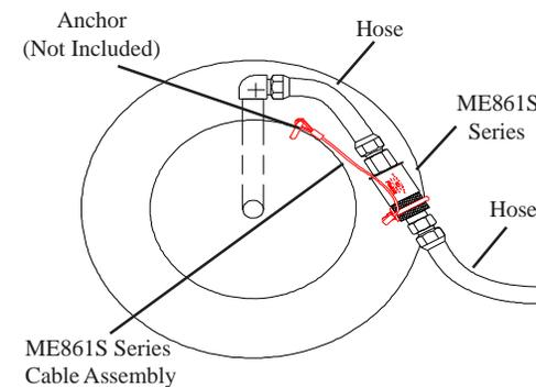
Use a short length of hose between the rigid piping and the inlet of the pull-away valve. Confirm the short length of hose is long enough to allow the pull-away valve to bear the brunt of any excessive tension load in the event of a pull-away.
