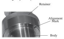
Mark the retainer and the FNPT body at the same point. Use these marks to realign the components during reassembly. Completely remove the setscrew from the retainer. Remove the retainer from the FNPT body. Then separate the FNPT body from the rest of the assembly and remove the seal ring and O-ring from the assembly.
