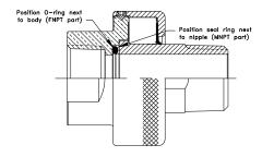
Lightly lubricate the replacement O-ring with a high quality lubricant (such as Dow Silicone or Lubriplate) and place the O-ring and seal ring into the FNPT body as shown. Position the O-ring next to the body and the seal ring next to the nipple during reassembly. Reassemble the FNPT body (with replacement O-ring and seal ring) to the retainer and tighten the assembly to align the marks made in the first step. This aligns the setscrew holes in the FNPT body and retainer. Reassemble the setscrew.
