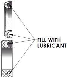
9. Install Stem O-Ring [3b], Female Adapter [3e], (2) V-Packs [3f], Bushing O-Ring (cut) [3h] and Male Adapter Bushing [3g] into Valve Shaft Gland [3a] as shown.
