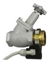
Tighten band around acme adapter and install mounting hardware through flange tabs as shown. Tighten mounting hardware using suitable wrench to secure interlock bracket to acme adapter.
