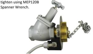
**NOTE:** Gap between sensor body and acme cap flange should be less than .062" as shown. If gap is greater than .062", sensor body may need to be adjusted forward to achieve proper sensing distance.
