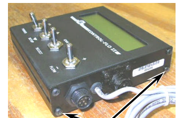
On the right side of the controller, remove the two screws on the bottom of the casing.
