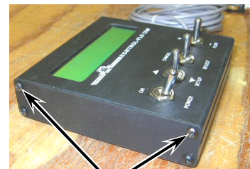
On the left side of the controller, remove the two screws on the top of the casing.
