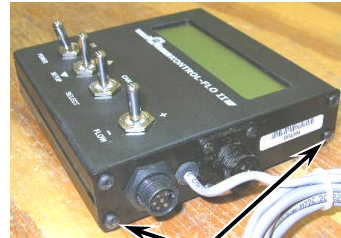
On the right side of the controller, remove the two screws on the bottom of the casing.
