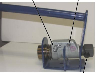
To mount a Hydrostat with this arrangement, install a Squibb-Taylor 2032-5000, 1-1/4" Adapter at the outlet of the FLO-MAX.
