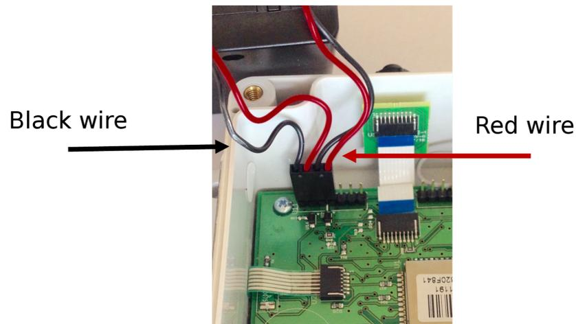
Orient the F100 so the Push Button is on your left. Insert the battery cable connector onto the seven pin connector so the black wire is on pin 1 (leftmost pin), and the red wire is on pin 4. Three pins remain uncovered as shown. The F100 will report when the battery cable is connected to the header.
