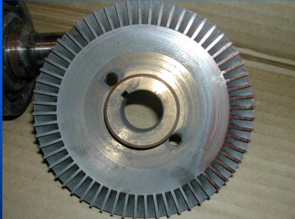
When an impeller is dis-colored such as shown in this photograph, the pump has operated “dry” or without liquid. This can be the cause of a seal failure. Inspect the system, bypass setting and operation to determine the cause of dry running. Note, the impeller may not be damaged if it can be properly shimmed and no “fins” are bent or damaged.
