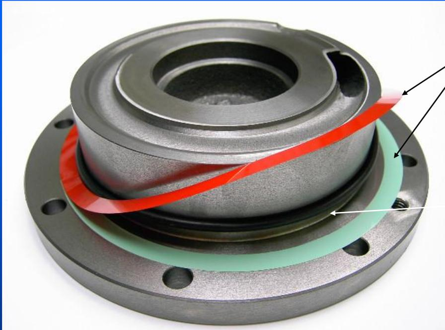
Shims are for adjusting impeller clearance.
