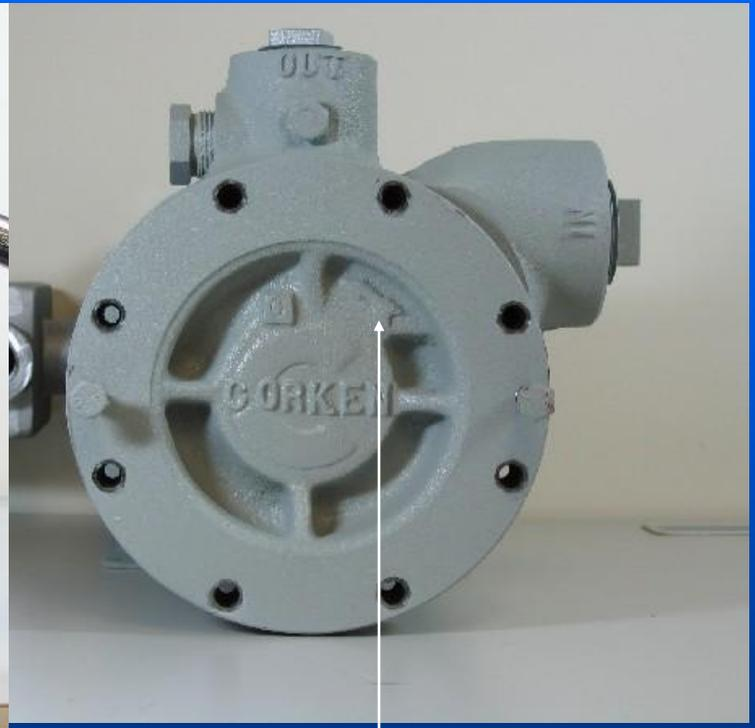
Remove the cover bolts and use two bolts to “push” off the cover if necessary. Note cover position and direction arrow. The pump operates “CCW” when facing the cover.
