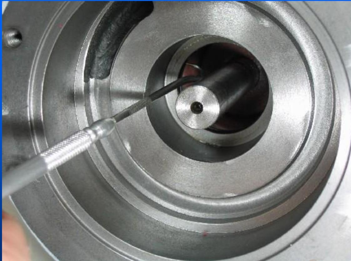
Remove the casing O-ring using a pick or probe. Once the O-ring is removed, clean the groove using a spray lubricant or air to remove any particles that may have fallen into the groove.
