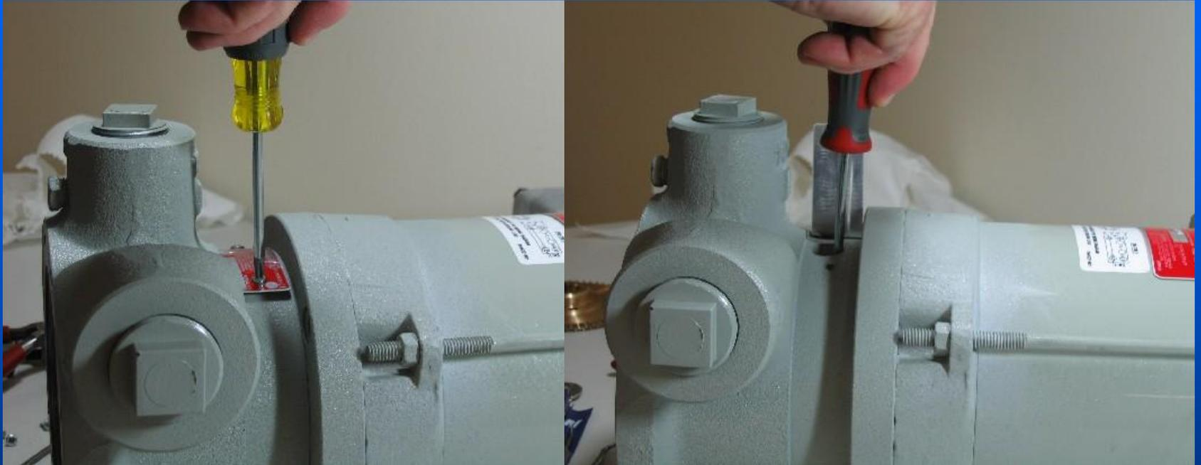
To remove the seal housing it is necessary to remove the nameplate. Then using a large flat blade screwdriver, pry outward on the housing. The screwdriver is prying on the grooves on the outside diameter of the housing. Holding up on the housing from the inside may assist in the removal.
